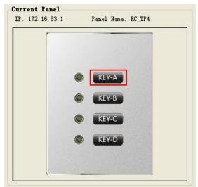
Select the key or lamp on the panel, and the information of the equipment under control in the function list will be filtered in accordance with the control type. The filter type shall be as follows:
