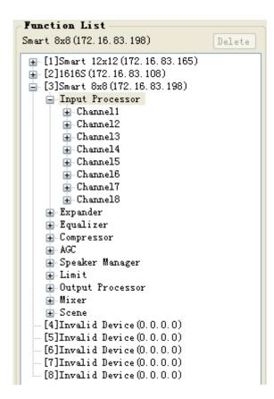
Select the panel in the "Target List" and "Set Current", and then select the equipment under control. Click the "Link", and the information of the associated equipment will be automatically displayed in the function list; in case of wrong choice, to select the root directory of corresponding equipment, and click the "Delete" button.
