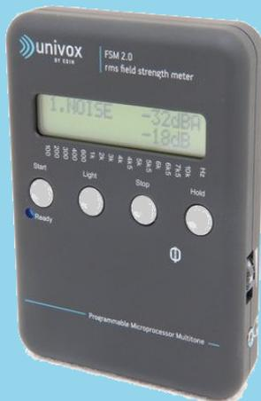
programmable, its mode of operation can be updated to reflect changes to the standard as they occur. The instrument has a clear, backlit, LCD display and steps through the required measurements in
