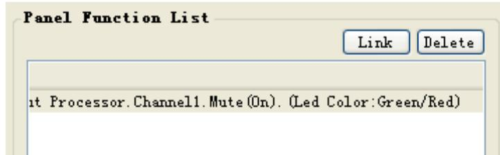
If the configuration of the indicator lamp is to be modified, the corresponding LED shall be selected in the current configuration panel, to reconfigure the related functions, or just change the color.
