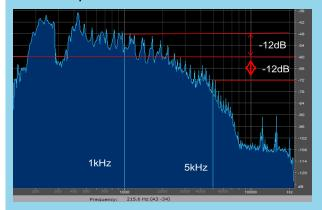
At 5kHz the signal level is approx. 24dB down on that at 1kHz. For every 12dB reduction in field strength the loop current is halved. This implies that at 5kHz, a  $\frac{1}{4}$  of the current is required compared to that at 1kHz which is  $\frac{1}{16}$ th of the power ( $P=I^2R$ ) so the system does not need to be capable of delivering full power all the way to 5kHz
