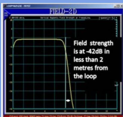
A SuperLoop system can provide excellent attenuation of the spill field
